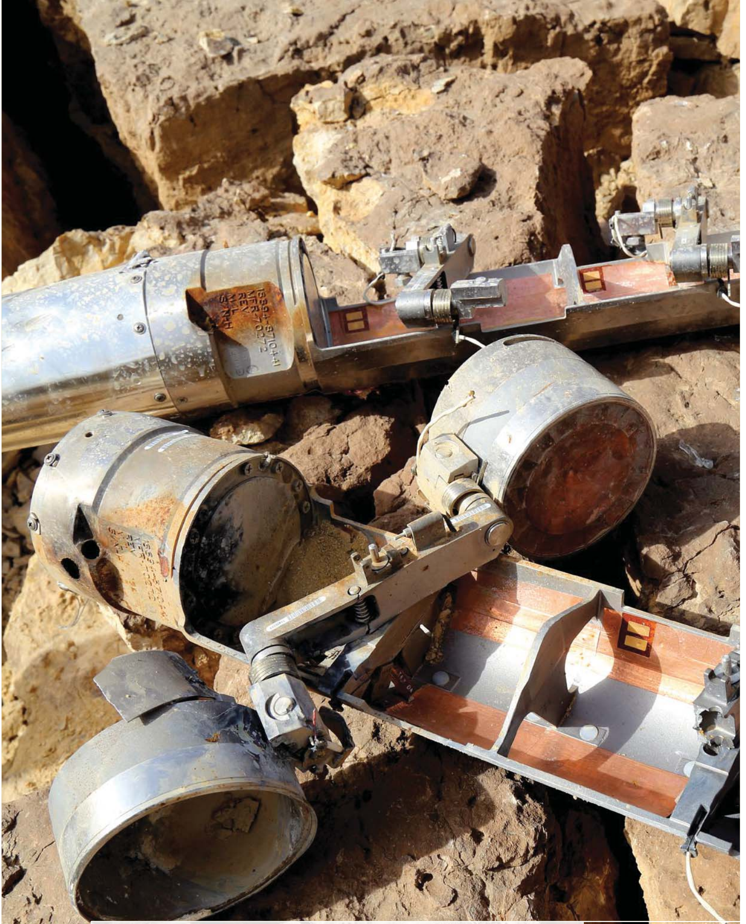
Two BLU-108 canisters disburSED from US-manufactured CBU-105 cluster munitions, one with two skeet (submunitions) still attached, found in the al-Amar area of al-Safraa in Saada governorate, northern Yemen after an attack on 27 April 2015. Under existing US policy, the CBU-105 is required to have a failure rate of less than 1%.
