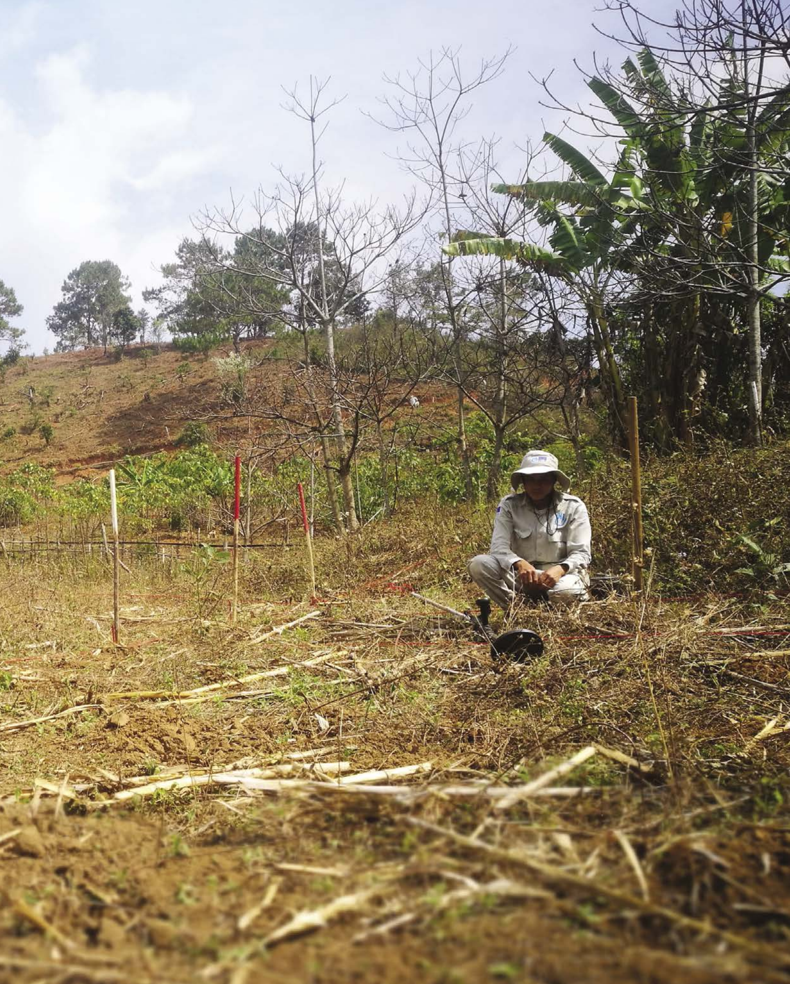
Humanity & Inclusion mine clearance operation in Laos. The deminer is equipped with a metal detector. To his right, the red pickets delimit the land and characterize the contamination.
